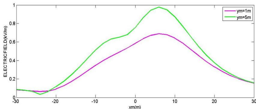
Fig.3 Electric Field at height 1m and 5m above ground.
