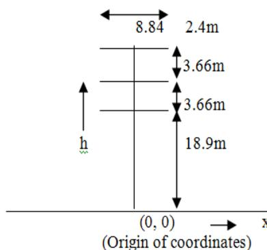
Fig.2 The 132kv tower structure
