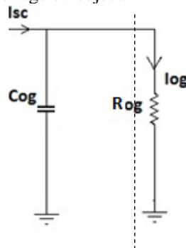
**Fig.1** Norton equivalent circuit.
