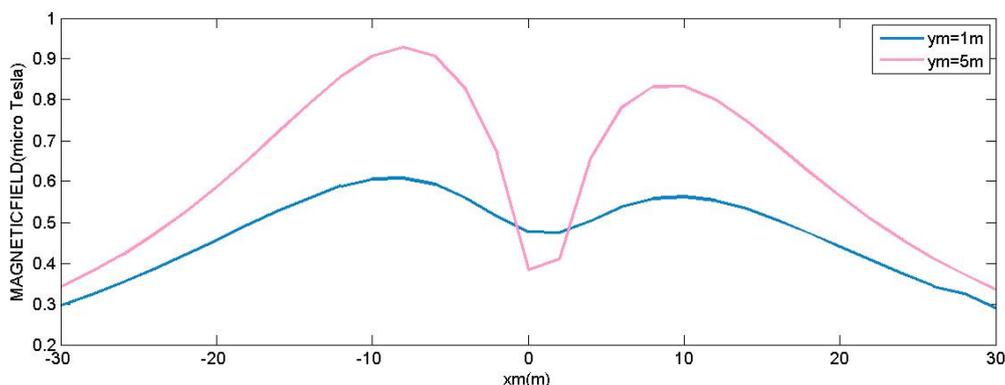
Fig.5 Magnetic field at 1m and 5m above ground.
